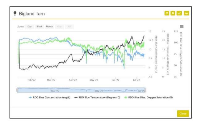
Control parameters are set within the database and warning notifications are automatically issued when readings fall outside set limits.
